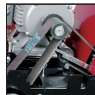
7 3VX V-belt drive from engine to center shaft
