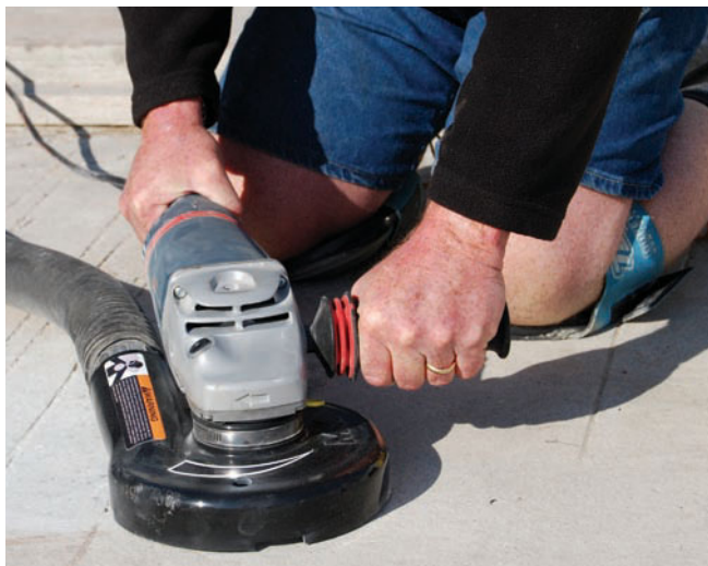
The IXL full shroud is designed for open areas.
