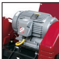
Baldor 20HP, 3 Phase, TEFC motor, providing 30ft-lb of torque
