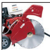
Cast aluminum hinged blade guard
