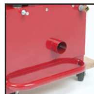
Vacuum port helps in dust control
