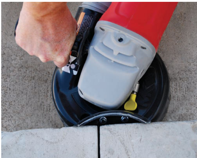
The IXL hinged shroud is designed for grinding against walls and edges.
